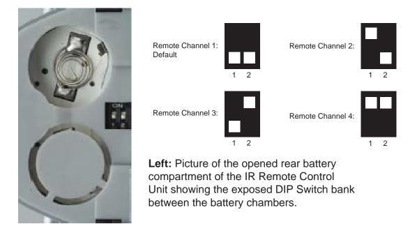
The IR channel selected on the IR Remote Control unit must match the IR channel assigned to the 4x2 Switcher for HDMI 1.3. For example, if you set both DIP switches on the remote to the down position (IR channel 1), you must set the 4x2 Switcher for HDMI 1.3 to use IR channel 1.
